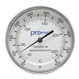
ProSense bi-metal dial thermometer, 5in diameter, 6in insertion length, 50 to 500 deg F/10 to 260 deg C, 1/2in male NPT process connection, center back, adjustable angle mount.
