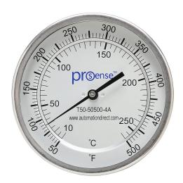
ProSense bi-metal dial thermometer, 5in diameter, 4in insertion length, 50 to 500 deg F/10 to 260 deg C, 1/2in male NPT process connection, center back, adjustable angle mount.
