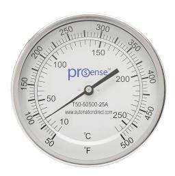
ProSense bi-metal dial thermometer, 5in diameter, 2-1/2in insertion length, 50 to 500 deg F/10 to 260 deg C, 1/2in male NPT process connection, center back, adjustable angle mount.
