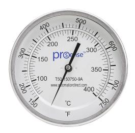
ProSense bi-metal dial thermometer, 5in diameter, 9in insertion length, 150 to 750 deg F/70 to 400 deg C, 1/2in male NPT process connection, center back, adjustable angle mount.
