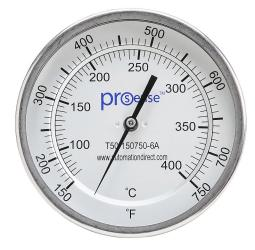
ProSense bi-metal dial thermometer, 5in diameter, 6in insertion length, 150 to 750 deg F/70 to 400 deg C, 1/2in male NPT process connection, center back, adjustable angle mount.
