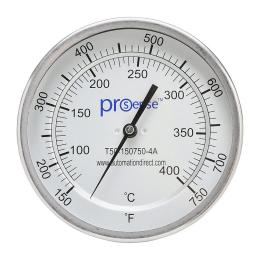
ProSense bi-metal dial thermometer, 5in diameter, 4in insertion length, 150 to 750 deg F/70 to 400 deg C, 1/2in male NPT process connection, center back, adjustable angle mount.
