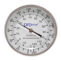
ProSense bi-metal dial thermometer, 5in diameter, 9in insertion length, 0 to 250 deg F/-18 to 120 deg C, 1/2in male NPT process connection, center back, adjustable angle mount.
