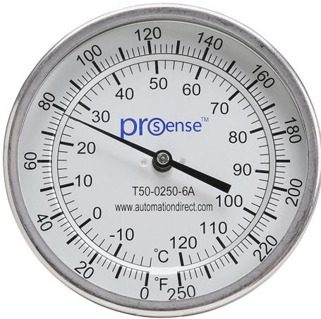
ProSense bi-metal dial thermometer, 5in diameter, 6in insertion length, 0 to 250 deg F/-18 to 120 deg C, 1/2in male NPT process connection, center back, adjustable angle mount.
