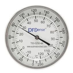
ProSense bi-metal dial thermometer, 5in diameter, 4in insertion length, 0 to 250 deg F/-18 to 120 deg C, 1/2in male NPT process connection, center back, adjustable angle mount.
