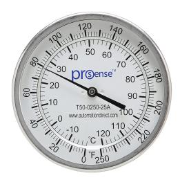
ProSense bi-metal dial thermometer, 5in diameter, 2-1/2in insertion length, 0 to 250 deg F/-18 to 120 deg C, 1/2in male NPT process connection, center back, adjustable angle mount.
