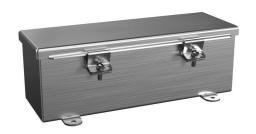
Wiegmann wiring trough, 4 x 4 x 12in (HxDxL), NEMA 1/4/4X/12, 304 stainless steel, No. 3 intermediate polished finish, single-door.
