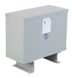
ACME general purpose transformer, encapsulated core, 15 kVA, 3-phase, 600 VAC Delta primary, 480Y/277 VAC secondary, 60 Hz, electrostatic shield, NEMA 3R, floor mount.
