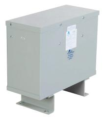
ACME general purpose transformer, encapsulated core, 15 kVA, 3-phase, 600 VAC Delta primary, 208Y/120 VAC secondary, 60 Hz, electrostatic shield, NEMA 3R, floor mount.
