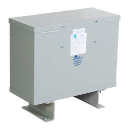
ACME general purpose transformer, encapsulated core, 15 kVA, 3-phase, 480 VAC Delta primary, 240/120 VAC Delta (center tap) secondary, 60 Hz, electrostatic shield, NEMA 3R, floor mount.
