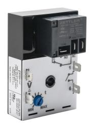
ProSense fleeting (single-shot) relay timer, 0.1 to 10 hours timing range, 24 VAC/VDC operating voltage, 30A contact rating, (1) SPDT timed relay output(s), surface mount, 1/4in male quick-connect terminal.
