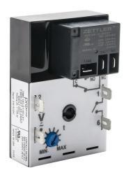
ProSense fleeting (single-shot) relay timer, 1 to 100 minutes timing range, 24 VAC/VDC operating voltage, 30A contact rating, (1) SPDT timed relay output(s), surface mount, 1/4in male quick-connect terminal.
