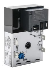
ProSense fleeting (single-shot) relay timer, 1 to 100 minutes timing range, 120 VAC/VDC operating voltage, 30A contact rating, (1) SPDT timed relay output(s), surface mount, 1/4in male quick-connect terminal.
