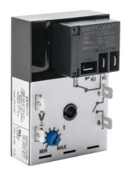
ProSense fleeting (single-shot) relay timer, 0.1 to 10 minutes timing range, 24 VAC/VDC operating voltage, 30A contact rating, (1) SPDT timed relay output(s), surface mount, 1/4in male quick-connect terminal.
