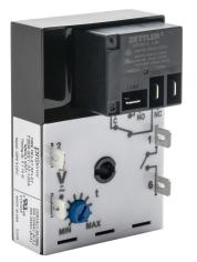
ProSense fleeting (single-shot) relay timer, 0.1 to 10 minutes timing range, 120 VAC/VDC operating voltage, 30A contact rating, (1) SPDT timed relay output(s), surface mount, 1/4in male quick-connect terminal.
