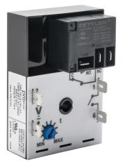
ProSense fleeting (single-shot) relay timer, 1 to 100 seconds timing range, 24 VAC/VDC operating voltage, 30A contact rating, (1) SPDT timed relay output(s), surface mount, 1/4in male quick-connect terminal.
