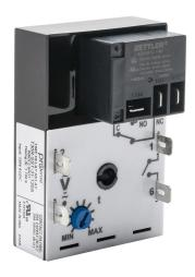
ProSense fleeting (single-shot) relay timer, 1 to 100 seconds timing range, 120 VAC/VDC operating voltage, 30A contact rating, (1) SPDT timed relay output(s), surface mount, 1/4in male quick-connect terminal.
