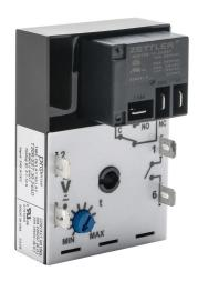
ProSense fleeting (single-shot) relay timer, 0.1 to 10 seconds timing range, 24 VAC/VDC operating voltage, 30A contact rating, (1) SPDT timed relay output(s), surface mount, 1/4in male quick-connect terminal.
