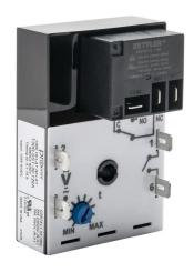
ProSense fleeting (single-shot) relay timer, 0.1 to 10 seconds timing range, 120 VAC/VDC operating voltage, 30A contact rating, (1) SPDT timed relay output(s), surface mount, 1/4in male quick-connect terminal.
