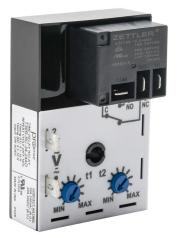
ProSense cyclic relay timer, 0.1 to 10 hours timing range, 24 VAC/ VDC operating voltage, 30A contact rating, (1) SPDT timed relay output(s), surface mount, 1/4in male quick-connect terminal.
