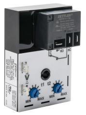
ProSense cyclic relay timer, 0.1 to 10 hours timing range, 120 VAC/ VDC operating voltage, 30A contact rating, (1) SPDT timed relay output(s), surface mount, 1/4in male quick-connect terminal.
