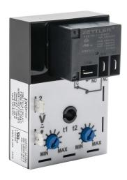
ProSense cyclic relay timer, 1 to 100 minutes timing range, 24 VAC/VDC operating voltage, 30A contact rating, (1) SPDT timed relay output(s), surface mount, 1/4in male quick-connect terminal.
