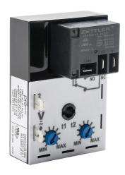
ProSense cyclic relay timer, 0.1 to 10 minutes timing range, 24 VAC/VDC operating voltage, 30A contact rating, (1) SPDT timed relay output(s), surface mount, 1/4in male quick-connect terminal.
