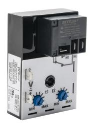
ProSense cyclic relay timer, 0.1 to 10 minutes timing range, 120 VAC/VDC operating voltage, 30A contact rating, (1) SPDT timed relay output(s), surface mount, 1/4in male quick-connect terminal.
