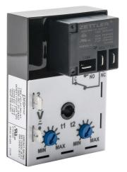
ProSense cyclic relay timer, 1 to 100 seconds timing range, 24 VAC/VDC operating voltage, 30A contact rating, (1) SPDT timed relay output(s), surface mount, 1/4in male quick-connect terminal.
