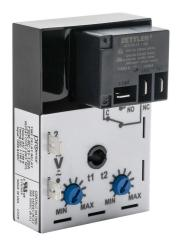
ProSense cyclic relay timer, 1 to 100 seconds timing range, 120 VAC/VDC operating voltage, 30A contact rating, (1) SPDT timed relay output(s), surface mount, 1/4in male quick-connect terminal.
