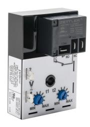
ProSense cyclic relay timer, 0.1 to 10 seconds timing range, 24 VAC/VDC operating voltage, 30A contact rating, (1) SPDT timed relay output(s), surface mount, 1/4in male quick-connect terminal.
