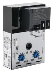
ProSense cyclic relay timer, 0.1 to 10 seconds timing range, 120 VAC/VDC operating voltage, 30A contact rating, (1) SPDT timed relay output(s), surface mount, 1/4in male quick-connect terminal.
