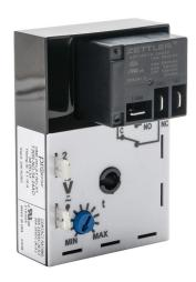
ProSense on-delay relay timer, 0.1 to 10 hours timing range, 24 VAC/VDC operating voltage, 30A contact rating, (1) SPDT timed relay output(s), surface mount, 1/4in male quick-connect terminal.
