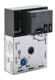
ProSense on-delay relay timer, 1 to 100 minutes timing range, 24 VAC/VDC operating voltage, 30A contact rating, (1) SPDT timed relay output(s), surface mount, 1/4in male quick-connect terminal.
