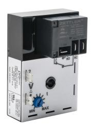
ProSense on-delay relay timer, 0.1 to 10 minutes timing range, 24 VAC/VDC operating voltage, 30A contact rating, (1) SPDT timed relay output(s), surface mount, 1/4in male quick-connect terminal.
