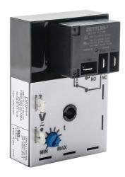
ProSense on-delay relay timer, 0.1 to 10 minutes timing range, 120 VAC/VDC operating voltage, 30A contact rating, (1) SPDT timed relay output(s), surface mount, 1/4in male quick-connect terminal.
