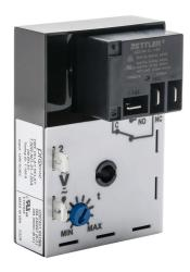
ProSense on-delay relay timer, 1 to 100 seconds timing range, 120 VAC/VDC operating voltage, 30A contact rating, (1) SPDT timed relay output(s), surface mount, 1/4in male quick-connect terminal.
