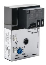
ProSense on-delay relay timer, 0.1 to 10 seconds timing range, 24 VAC/VDC operating voltage, 30A contact rating, (1) SPDT timed relay output(s), surface mount, 1/4in male quick-connect terminal.
