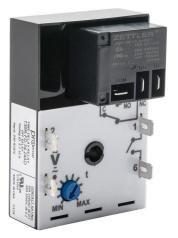
ProSense off-delay relay timer, 0.1 to 10 hours timing range, 24 VAC/VDC operating voltage, 30A contact rating, (1) SPDT timed relay output(s), surface mount, 1/4in male quick-connect terminal.
