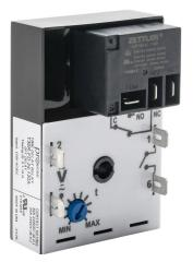
ProSense off-delay relay timer, 0.1 to 10 hours timing range, 120 VAC/VDC operating voltage, 30A contact rating, (1) SPDT timed relay output(s), surface mount, 1/4in male quick-connect terminal.
