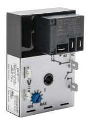
ProSense off-delay relay timer, 1 to 100 minutes timing range, 24 VAC/VDC operating voltage, 30A contact rating, (1) SPDT timed relay output(s), surface mount, 1/4in male quick-connect terminal.
