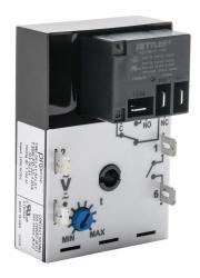
ProSense off-delay relay timer, 1 to 100 minutes timing range, 120 VAC/VDC operating voltage, 30A contact rating, (1) SPDT timed relay output(s), surface mount, 1/4in male quick-connect terminal.
