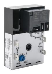
ProSense off-delay relay timer, 0.1 to 10 minutes timing range, 24 VAC/VDC operating voltage, 30A contact rating, (1) SPDT timed relay output(s), surface mount, 1/4in male quick-connect terminal.
