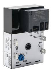
ProSense off-delay relay timer, 0.1 to 10 minutes timing range, 120 VAC/VDC operating voltage, 30A contact rating, (1) SPDT timed relay output(s), surface mount, 1/4in male quick-connect terminal.
