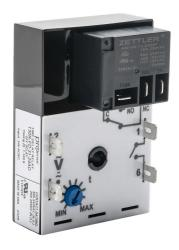
ProSense off-delay relay timer, 1 to 100 seconds timing range, 24 VAC/VDC operating voltage, 30A contact rating, (1) SPDT timed relay output(s), surface mount, 1/4in male quick-connect terminal.
