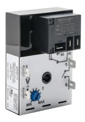
ProSense off-delay relay timer, 1 to 100 seconds timing range, 120 VAC/VDC operating voltage, 30A contact rating, (1) SPDT timed relay output(s), surface mount, 1/4in male quick-connect terminal.
