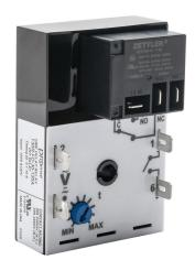
ProSense off-delay relay timer, 0.1 to 10 seconds timing range, 120 VAC/VDC operating voltage, 30A contact rating, (1) SPDT timed relay output(s), surface mount, 1/4in male quick-connect terminal.
