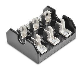
Bussmann fuse block, accepts T fuses, 30A, 300V, 3-pole, 18-10 AWG copper only, screw with pressure plate, panel mount.
