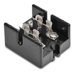
Bussmann fuse block, accepts T fuses, 30A, 300V, 2-pole, 18-10 AWG copper only, screw with pressure plate, panel mount.
