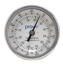
ProSense bi-metal dial thermometer, 3in diameter, 6in insertion length, -40 to 160 deg F/-40 to 70 deg C, 1/2in male NPT process connection, center back mount.
